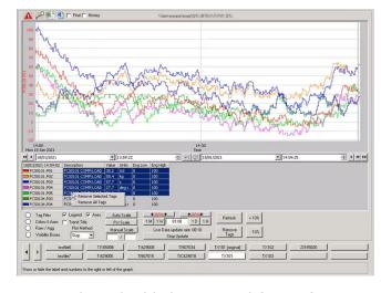
to years of historical data that can be called up from a DCS console and added to a trend for performance comparison or to understand and visualise any changes to equipment performance over time.
